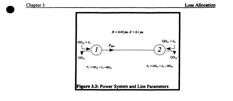
The two bus system shown in figure (3.3) is used to investigate the nature of the generalized loss allocation procedure and to show the effect of the choice of generator on total and contractual losses. Recall that  $\overline{L_i}$  represents the amount of generation at bus i dedicated to transmission losses. Four different cases are investigated using the MW load matrix,
